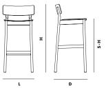
DIMENSIONS L 457 x D 465 x H 953 mm L 17.9 x D 18.3 x H 37.5 "
