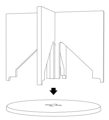
Place top plate on the floor and press legs inside. If needed rotate legs 90  $^{\rm o}$  clockwise until perfect fit!
