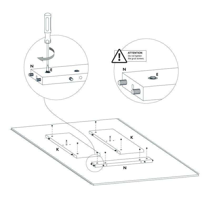
ATTACH THE LEG PANELS TO CROSS RAIL AND TIGHTEN THE GRUB SCREWS BY USING A SCREWDRIVER.
