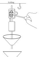
Place the ring on the connection box and on the cord onto the hook that is mounted to the ceiling. Push the canopy up to the ceiling.
